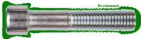
Figure D.3 - Illustration of typical distribution of coating thickness on bolt resulting from electroplating process
